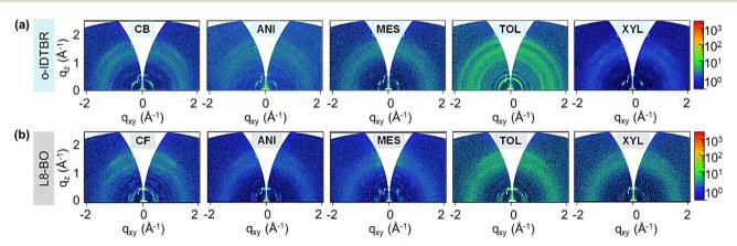
Fig. 4 Two-dimensional grazing incident wide angle X-ray scattering (2D-GIWAXS) spectra of (a) o-IDTBR and (b) L8-BO films processed from different solvents.
