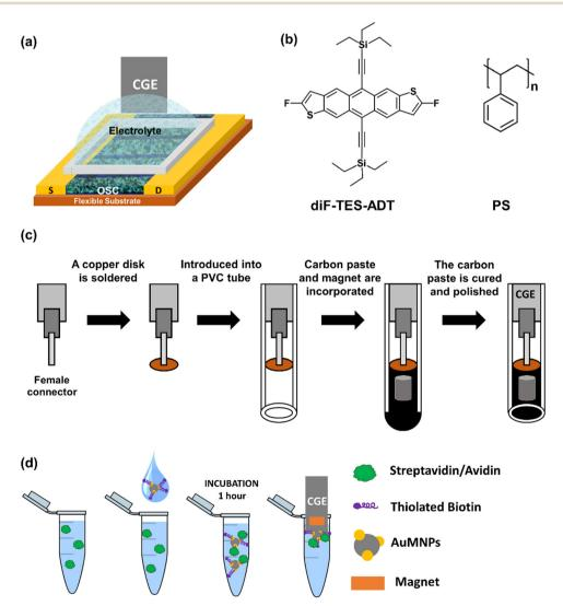
Fig. 1 (a) Scheme of the EGOFET structure. (b) Molecular structure of diF-TES-ADT and PS. (c) Schematic illustration of magnetic CGE fabrication. (d) Scheme of the sensing protocol.
