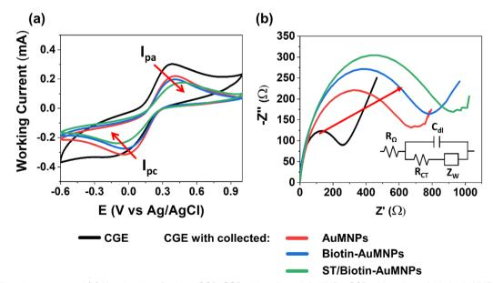
Fig. 2 (a) Cyclic voltammetry and (b) Nyquist plots for bare CGE, CGE with collected AuMNPs, CGE with collected biotin-AuMNPs and CGE with collected ST/biotin-AuMNPs ([ST] =  $10^{-10}$  M). All the electrochemical measurements were carried out in a three-electrode configuration using a 0.1 M KCl aqueous solution containing 10 mM [Fe(CN)<sub>6</sub>]<sup>3-/4-</sup> as redox probe.
