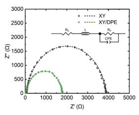
Fig. 3 Nyquist plot of solar cells fabricated with and without DPE. Experimental data (dots) and best fits (dash lines). Inset: equivalent circuit used to fit the experimental data.
