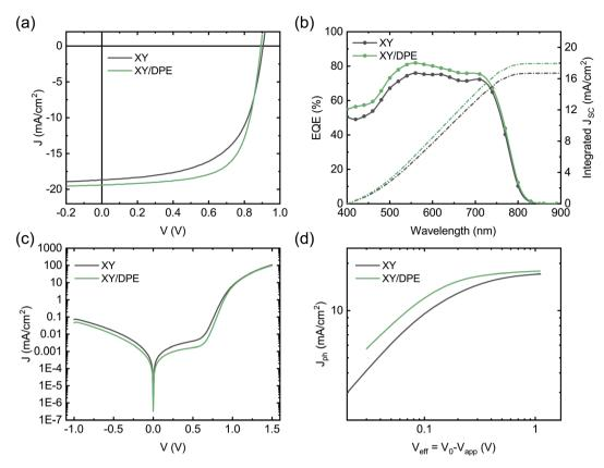
Fig. 2 Electrical characteristics of optimized solar cells, fabricated by spin coating from a o-xylene solution without additive and with 3 wt% of DPE: (a) J-V curves under illumination (AM 1.5, 100 mW cm<sup>-2</sup>); (b) EQE spectra and integrated  $J_{sc}$ ; (c) J-V curves in dark condition; (d)  $J_{ph}$  as a function of  $V_{eff}$ .
