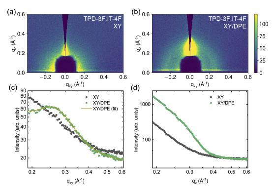
Fig. 5 2D GIWAXS data and cuts of measurements on TPD-3F:IT-4F blend films cast with and without the addition of DPE: 2D false-color maps for a blend film without additive (a) and with additive (b); corresponding in-plane (c) and out-of-plane (d) line cuts.
