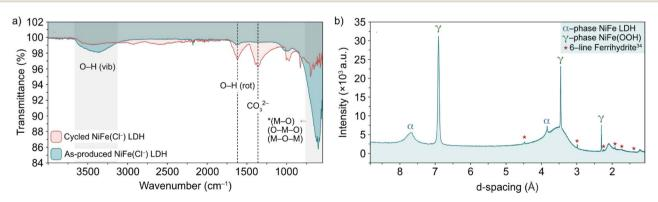
Fig. 6 (a) FT-IR spectra of pre-cycled (black line) and post-cycled (red line) Cl<sup>-</sup>-intercalated NiFe LDH and (b) XRD pattern for NiFe LDH after 200 cycles between 1.02–1.62 V vs. RHE at 5 mV s<sup>-1</sup>. The  $\alpha$ -NiFe LDH and  $\gamma$ -NiFeOOH phases are labelled, as well as a ferrihydrite signal at low dspacing.1
