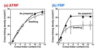
Fig. 1 The effect of the cross-linker content on the cross-linking density of the PNIPAAm gels (●, as-prepared; ○, swollen) synthesized via ATRP (a) and FRP (b). The cross-linking densities were determined from the compression modulus
