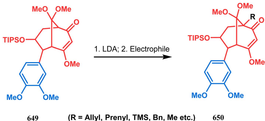
Scheme 147 Metallation at the bridgehead position during the synthesis of the bicyclic core of garsubellin A.
