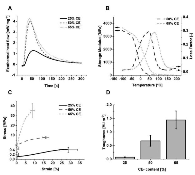
Fig. 4 Photo-DSC results for the formulations containing aromatic monofunctional 5P-S and bifunctional epoxide CE in varying concentrations at 110 °C and with 1 wt% IC 290 as photoinitiator (A), storage moduli G' and loss factors  $\tan \delta$  (B), representative tensile testing curves and mean stress and strain at break values (C) and toughness (D) of specimens obtained from the same formulations at 110 °C.
