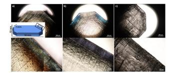
Fig. 5 Optical microscopy images of transparent bulk-cured samples for (a) 0, (b) 35 and (c) 75 wt% 5P-S content crosslinked with the diepoxide CF
