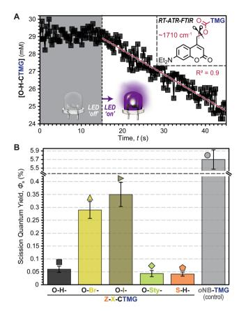
Fig. 5 Estimating photouncaging quantum yields. (A) Carbamate bond scission was tracked and quantified using RT-FTIR in an attenuated total reflectance (ATR) configuration during violet LED irradiation, using 0.5 mol% photocages in DODT. (B) Bar graph showing bond scission quantum yields ( $\phi_s$ ) for each derivative. Dashed line represents break in data for clarity. Averages were calculated from a minimum of three samples and error bars represent  $\pm 1$  standard deviation from the mean.
