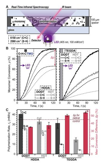
Fig. 3 Photopolymerization resin optimization. (A) Illustration of the transmission real-time Fourier transform infrared (RT-FTIR) spectroscopy setup used to monitor monomer to polymer conversion  $(\rho)$ during LED irradiation. (B) Photopolymerization kinetics as a function of diacrylate and dithiol composition. (C) Maximum polymerization rate  $(r_p)$ and difference in maximum C=C and S-H conversion  $(\Delta \rho)$  for different resin compositions. Dashed line represents  $\Delta
