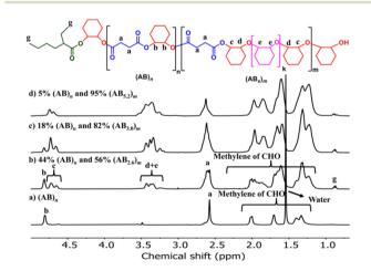
Fig. 2  $\,^{1}$ H NMR spectra (600 MHz, CDCl<sub>3</sub>, 30 °C) of the copolymer from ROCOP of SA and CHO having different AB and AB $_{x}$  components.
