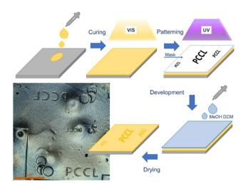
Fig. 7 Schematic procedure and positive-tone photopatterns inscribed in a thiol-acrylate photopolymer containing PDS-triflate as latent catalysts.
