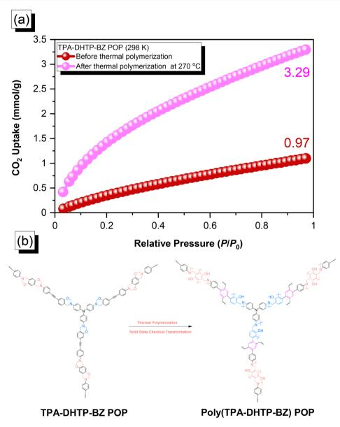
Fig. 9 (a) CO<sub>2</sub> uptake of the TPA-DHTP-BZ POP and poly(TPA-DHTP-BZ) POP. (b) Corresponding chemical structures before and after the thermal ROP.
