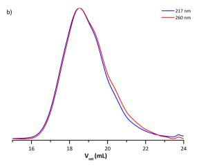
**Fig. 5** (a) Molar mass distributions of dry extracts for latexes E4BMDO (red), E5BMDO (blue), E1BMDO (green) and EMMA1 (black) (Table 1). (b) UV chromatograms from SEC-THF analysis at 217 nm (blue) and 260 nm (red) for the dried latex E5BMDO.
