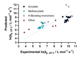
Fig. 2 The predicted versus experimental values of the  $ln(k_p)$  at 25 °C for a dataset n = 41 using the leave one out cross validation on a linear regression. Predictions are determined using Mr, inductive effects, DP, BPK, MPK, and GFE ( $r^2 = 0.631$ , RME = 1.167).
