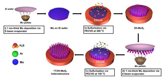
Scheme 1 Synthesis steps of the vertical stacking of 1T- and 2H-MoS<sub>2</sub> on Si substrates using a 13.56 MHz ICP plasma process.
