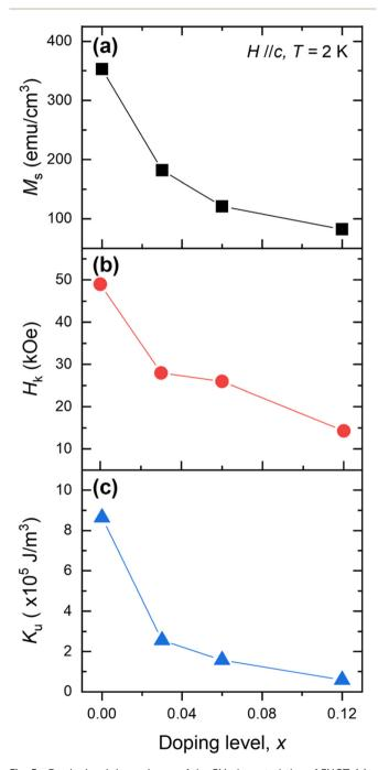
Fig. 5 Dopinglevel dependence of the FM characteristics of FNGT. (a) x dependence of the saturation magnetization ( $M_s$ ) of FNGT. (b) x dependence of the anisotropy field  $(H_k)$  of FNGT. (c) x dependence of the anisotropy energy ( $K_u$ ) of FNGT. All data are measured with H//c at 2 K.
