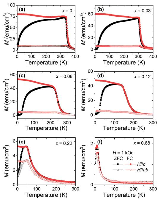
Fig. 3 Temperature-dependentmagnetization curves of FNGT. (a-f) Field cooling (FC) and zero-field cooling (ZFC) temperature-dependent magnetization (M-T) curves of FNGT with x = 0-0.68 with H//c and H//ab, H = 1 kOe.
