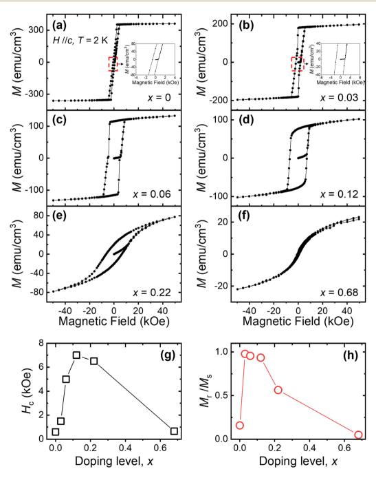
Fig. 4 Hysteresisloop of FNGT at 2 K. (a–f) Hysteresis loop of FNGT with x = 0-0.68. The field range is  $\pm 50$  kOe. The insets in (a and b) are the magnification of the red-dashed area. (g) x dependence of coercive fields  $(H_c)$ . (h) x dependence of the ratio of remanent magnetization  $(M_r)$  to saturation magnetization ( $M_s$ ). Every  $H_c$  and  $M_r/M_s$  is obtained from Fig. 4a–f. All data are measured with H//c at 2 K.
