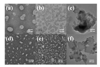
Fig. 9 TEM images of molecule  $H_1 \subset G$  (c/c = 4:1) obtained from  $CHCl_3/DMSO$  (v/v = 19:1) solutions after (a) 1 h, (b) 4 h and (c) 24 h. TEM images of molecule  $H_2 \subset G$  (c/c = 4:1) obtained from CHCl<sub>3</sub>/DMSO (v/v = 19:1) solution after (d) 1 h, (e) 4 h and (f) 24 h.
