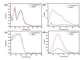
Fig. 1 The absorption spectra of (a)  $H_1$  and (c)  $H_2$ , and emission (excited at 298 nm, Ex bandwidth: 2.5 nm; Em bandwidth: 5 nm) spectra of (b)  $H_1$  and (d)  $H_2$  in DMSO and  $H_2$ O/DMSO (v/v = 19:1) solutions (3.03  $\times$  10<sup>-6</sup> mol L<sup>-1</sup>).
