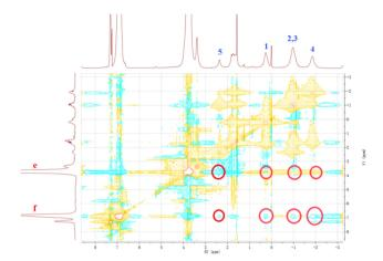
Fig. 7 <sup>1</sup>H-<sup>1</sup>H NOESY NMR spectrum (500 MHz) of the complex of G with H<sub>3</sub> at a 1:4 molar ratio in CDCl<sub>3</sub> at 25 °C.
