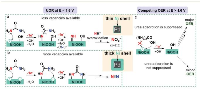
Fig. 3 The effect of the tensile strain on the UOR mechanistic pathways and competing OER. (a and b) A schematic illustration of the proposed pathways for UOR to  $NO_x$  products (a)  $N_2$  (b) on the NiOOH surface of Pd@Ni NCs with thin shell (a) and thick shell (b) at E < 1.6 V vs. RHE. (c) A schematic illustration of the competition between UOR and OER on the NiOOH surface of Pd@Ni NCs with thin shell and thick shell at E > 1.6 V vs.
