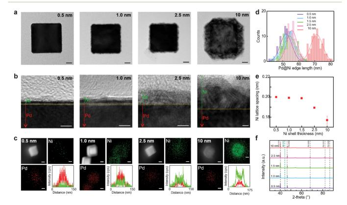
Fig. 1 Structural analysis of Pd@Ni NCs with different Ni thickness (0.5, 1.0, 2.5, and 10 nm): TEM images (a), HRTEM images (b), elemental mapping (c), edge length distribution (d), Ni lattice spacing (e), and XRD spectra (f). In (b), the dotted green line is a guide for Ni layer, and the dotted red line is a guide for Pd layer. In (c), Ni is indicated in green, and Pd is indicated in red. Scale bars: 10 nm in (a), 2 nm in (b), and 20 nm in (c).
