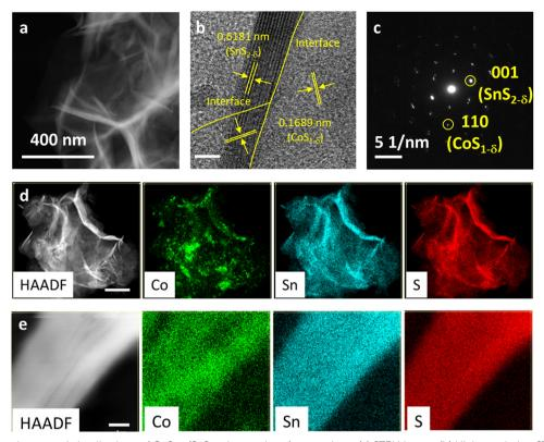
Fig. 1 Microscopic and structural visualizations of  $CoS_{1-\delta}/SnS_{2-\delta}$  hetero-interface catalysts. (a) STEM image. (b) High-resolution STEM (HRTEM) image hetero-interface of  $CoS_{1-\delta}$  and  $SnS_{2-\delta}$ . Scale 5 nm. (c) SAED pattern. (d) HAADF-STEM image and the corresponding maps for Co, Sn, and S. Scale 200 nm. (e) HAADF-STEM image and the corresponding maps at a specified edge site region for Co, Sn, and S with  $CoS_{1-\delta}/SnS_{2-\delta}$  phase. Scale 5 nm.
