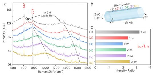
Fig. 6 WGM cavity sensing mechanisms: optical resonance coupling. (a) Raman spectra collected from a  $ZnO_{1-x}$  cavity ( $d \approx 2 \mu m$ ) with a side length gradient. (b) Schematics of the  $ZnO_{1-x}$  cavity with side length gradient. (c) The Raman intensity ratio columns of  $I_{612}/I_{773}$  from different sites.
