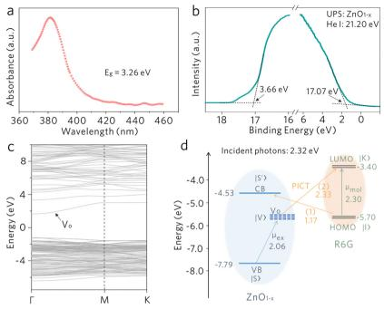
Fig. 4 WGM cavity sensing mechanism: photoinduced charge transfer. (a) UV-vis spectrum of  $ZnO_{1-x}$ . (b) UPS spectrum of  $ZnO_{1-x}$ . (c) DFT calculations of the electronic band structure of ZnO<sub>1-x</sub>, Vo represent the oxygen-vacancy-associated defect level. (d) Energy level diagram of the R6G molecule on  $ZnO_{1-x}$  under the excitation of 532 nm (2.32 eV)
