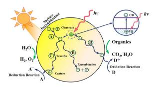
Fig. 1 Diagram of the photocatalytic principle.
