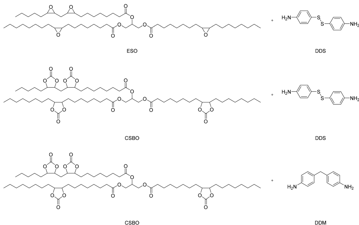
Fig. 22 Reaction scheme for obtaining poly-oil (ESO-DDS) and partially bio-based NIPUs (CSBO-DDM and CSBO-DDS).
