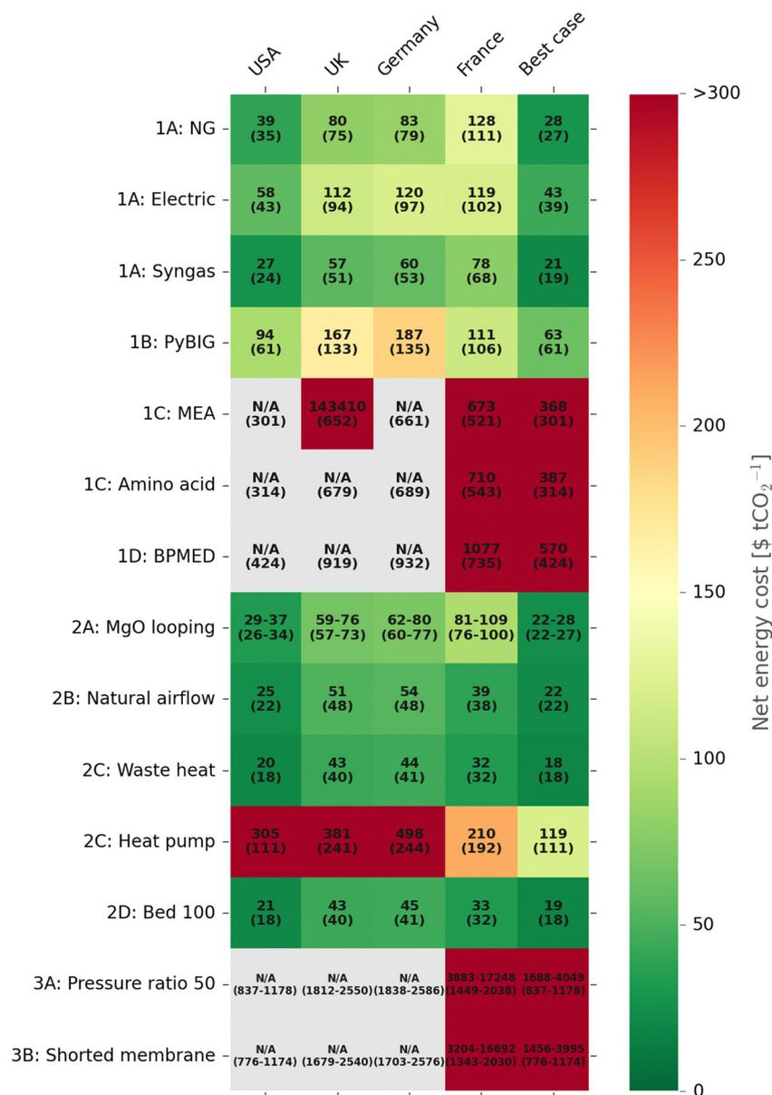
Fig. 3 Net energy and gross energy (in brackets) costs in USD per tCO<sub>2</sub>. The costs are provided for the 14 DAC configurations and for 5 electricity mix cases: USA, UK, Germany, France, and 'best case'. 'N/A' denotes net positive emissions due to an emissions factor (*i.e.*, amount of CO<sub>2</sub> emitted over amount of CO<sub>2</sub> captured) of >1 (see Section S2 in ESI†).
