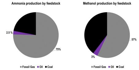
Fig. 8 Ammonia (left) and methanol (right) production by feedstock in 2013 according to Levi and Cullen.<sup>8</sup>
