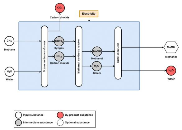
Fig. 2 Conventional production process for methanol synthesis from natural gas over a CuO/ZnO/Al<sub>2</sub>O<sub>3</sub> catalyst. Coal and oil can similarly be used as fossil feedstocks for coal gasification and partial oxidation for syngas production, respectively. Adapted from Adnan and Kibria.<sup>20</sup>
