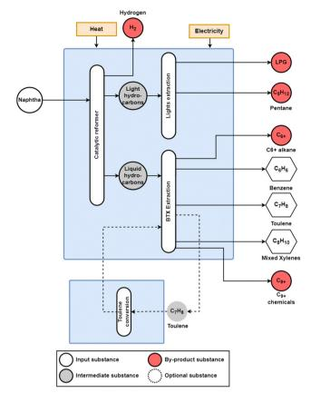
Fig. 4 Conventional naphtha catalytic reforming (CRR) process. The main products from this process are the BTX aromatics, and the by-products include pentane, C<sub>6+</sub> alkane, liquefied petroleum gas (LPG), and C<sub>9+</sub> chemicals, with an optional toluene conversion route to increase benzene and xylene yields. Adapted from Jiang et al. 26
