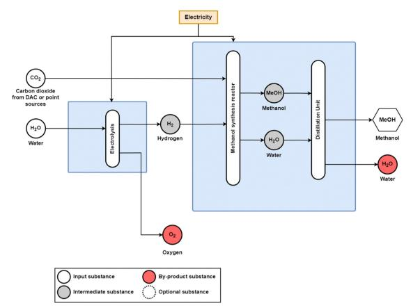
Fig. 12 Power-to-methanol process diagram with e-hydrogen supplied by water electrolysis and CO<sub>2</sub> being supplied by direct air capture (DAC) or industrial point sources. In this study,  $CO_2$  from DAC is assumed. The catalyst for the methanol synthesis reactor is  $CuO/ZnO/Al_2O_3$ . Adapted from Adnan and Kibria<sup>20</sup> and Bos et al.<sup>64</sup>
