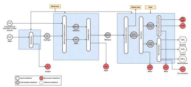
Fig. 14 Power-to-methanol-to-aromatic process diagram. Methanol synthesis occurs over a CuOZnO/Al<sub>2</sub>O<sub>3</sub> catalyst, and methanol aromatisation occurs over a HZSM-5 catalyst. Adapted from Jiang et al.<sup>26</sup>
