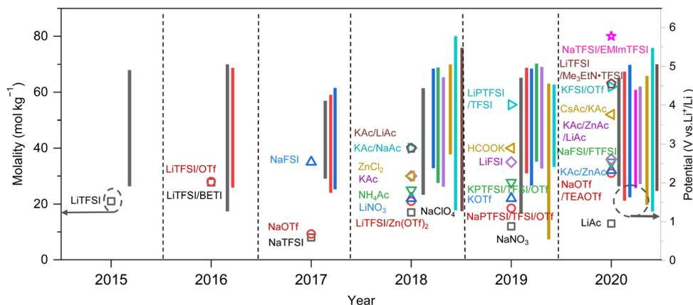
Fig. 2 Development of highly concentrated aqueous electrolytes in recent years: concentration (scattered points) and corresponding ESW (bars) of each electrolyte.<sup>12,24–51</sup>
