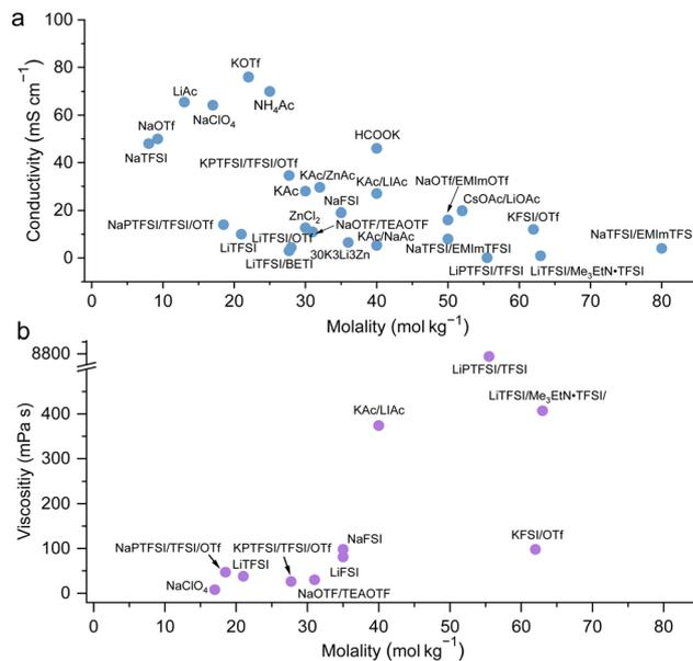
Fig. 8 Ion conductivity (a) and viscosity (b) for representative highly concentrated aqueous electrolytes, respectively.<sup>12,24–29,32–50</sup>
