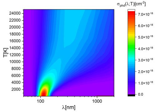
Fig. 3 The surface plot of average cross-section for photodissociation, against  $\lambda$  and T, of  $H_2^+$  molecular ion. The dataset is obtained in Srećković et al.<sup>45</sup>
