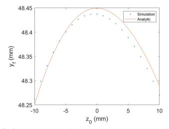
Fig. 6 Impact position  $y_f$  as a function of the source position  $z_0$ , for  $\varepsilon_{\text{max}}$  =  $1.8\ {\rm eV}.$  We used an electron beam starting from the origin with velocity on the y axis only, which corresponds to a kinetic energy of 1 eV. We observe very small deviations (less than 0.041%) that practically can be neglected, since they are smaller than the detector's resolution.
