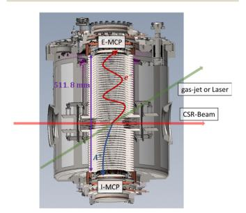
Fig. 1 A schematic illustration of the CSR-ReMi. In this illustration the stored ion beam passes through the instrument from left to right (along the direction indicated by the red arrow), and is crossed by either a neutral gas jet or by laser (along the direction indicated by the green arrow). The resulting electrons are accelerated upwards and imaged on the E-MCP detector, while the resulting cationic fragments are accelerated in the opposite direction and imaged on the I-MCP detector.
