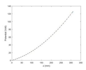
Fig. 3 Comparison of the numerically calculated potential along the  $\hat{z}$ axis (for the same value of  $\varepsilon_{\text{max}}$  used in Fig. 2), as a function of z, to the analytical formula (eqn (2)). Here z = 0 corresponds to the center of the interaction zone. We observe small deviations (up to 1.2%) from the analytical potential only at small distances (<15 mm) from the detector.
