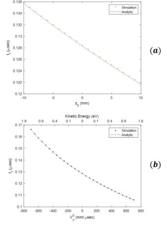
Fig. 5 (a) Time-of-flight for a beam of electrons starting from different positions along the  $\hat{z}$  axis between  $z_0 = -10$  mm to  $z_0 = 10$  mm, for  $x_0 = -10$  $y_0$  = 0, and for  $\varepsilon_{\text{max}}$  = 1.8 eV. (b) Time-of-flight for a beam of electrons starting from the origin with velocity on z axis only for  $\varepsilon_{\text{max}}$  = 1.8 eV.
