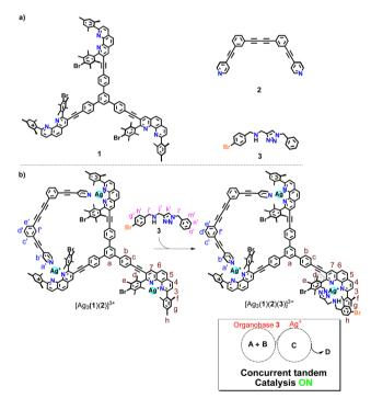
Scheme 1 (a) Chemical structure of ligands 1-3. (b) Transformation of the three- into the four-component dual-catalyst machinery. Both organobase 3 and the silver(ı) centers are liberated due to the sliding motion in  $[Ag_3(1)(2)(3)]^{3+}$ , which enables concurrent tandem catalysis. A & B represent the substrates, C denotes the intermediate product and D the final product of the concurrent tandem reaction.
