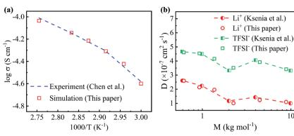
Fig. 2 (a) Simulated conductivity and (b) diffusion coefficients of PEO-LiTFSI electrolytes and comparison with the previous experimental and simulated results. 45,46
