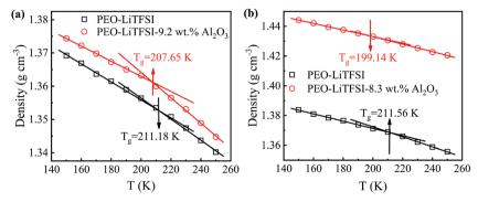
Fig. 7 Densities of the SPE at different temperatures for (a) the SC system and (b) the LC system.
