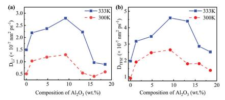
Fig. 3 Diffusivities of (a) Li<sup>+</sup> and (b) TFSI<sup>-</sup> at different temperatures in the SC system.
