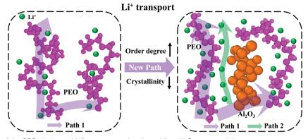
Structural changes of the PEO chains and Li<sup>+</sup> transport paths after adding Al<sub>2</sub>O<sub>3</sub> nanoparticles
