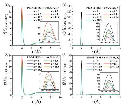
Fig. 6 RDFs for (a) Li<sup>+</sup>-O(PEO) at 333 K, (b) Li<sup>+</sup>-O(TFSI) at 333 K, (c) Li<sup>+</sup>-O(PEO) at 300 K, and (d) Li<sup>+</sup>-O(TFSI) at 300 K in the LC systems. The insets show the enlargement of the first coordination shell
