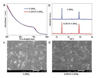
Fig. 1 UV-vis (a) and XRD (b) spectra of CsPbl<sub>3</sub> and 0.2PAN-CsPbl<sub>3</sub> thin films, and top-surface SEM images of CsPbI<sub>3</sub> (c) and 0.2PAN-CsPbI<sub>3</sub> films (d). Scale bar, 1 um.
