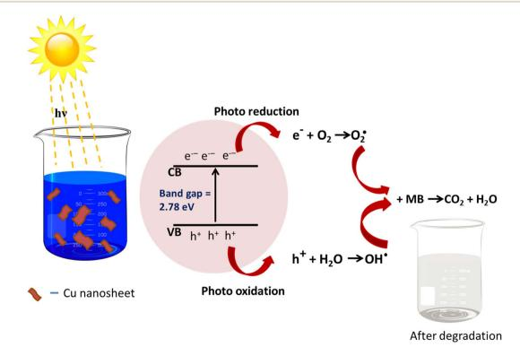
Fig. 12 Schematic representing the MB dye degradation mechanism using Cu nanosheets.
