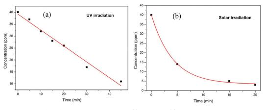
Fig. 10 Reaction kinetics model fitting for MB dye degradation under (a) UV light and (b) solar light irradiation.
