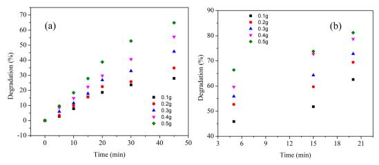
Degradation of MB dye with recycled Cu nanosheet powder under (a) UV light and (b) solar light irradiation.
