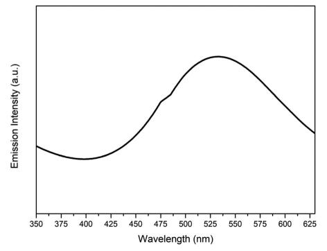
Fig. 11 Photoluminescence spectra of Cu nanosheets.
