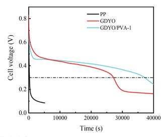
Fig. 5 SDC of the supercapacitors with different membranes when the electrolyte is a 1 M H<sub>2</sub>SO<sub>4</sub> and 0.5 M KI mixture.
