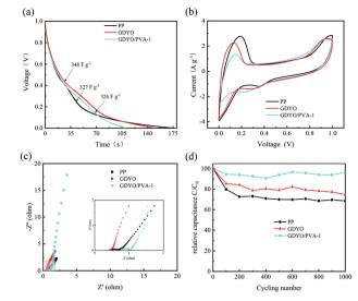
Fig. 4 AEESEs based on the different membranes membrane: PP; GDYO membrane and GDYO/PVA-1 membrane) when the electrolyte is a 1 M H<sub>2</sub>SO<sub>4</sub> and 0.5 M KI mixture (a) Charge-discharge curves at a current density of 1 A g<sup>-1</sup>. (b) CVs at a scan rate of 10 mV s<sup>-1</sup> (c) EIS analysis. (d) Cycling stability at a current density of 1 A  $g^{-1}$ .
