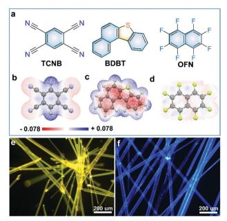
Fig. 1 (a) The molecular structures of TCNB, BDBT, and OFN. ESP maps of (b) TCNB, (c) BDBT, and (d) OFN. Fluorescence microscopy (FM) images of (e) BDBT-TCNB cocrystals and (f) BDBT-OFN cocrystals.
