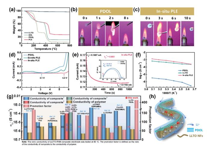
Fig. 2 Physicochemical properties of DOL and different electrolytes. (a) TGA curve. Combustion tests of (b) PDOL and (c) PLE electrolytes. (d) LSV curve, and (e) current-time profile of the Li|In-situ PLE|Li symmetrical cell after applying a DC voltage of 10 mV. (f) Ionic conductivity under different temperatures. (g) Comparisons of the ionic conductivity with different solid electrolytes. (h) Schematic diagram of the bi-phase ion conduction within the In-situ PLE.
