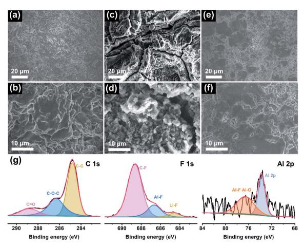
Fig. 4 Interfacial characterizations of the anode surface. SEM images of Li metal after 50 cycles with (a and b) PDOL electrolyte, (c and d) Ex-situ PLE and (e and f) In-situ PLE. (g) XPS spectra of the cycled Li anode from the symmetric battery using In-situ PLE.
