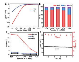
Fig. 2 Electrocatalytic  $CO_2RR$  performance of the SU-101 NRs. (a) LSV curves in  $N_2$ - (blue line) or  $CO_2$ - (red line) saturated 0.5 M KHCO $_3$  aqueous solution at a scan rate of 5 mV s $^{-1}$ . (b) FEs of  $H_2$ , CO and HCOO $^-$  at different applied potentials. (c) Partial current densities of  $H_2$ , CO and HCOO $^-$ . (d) Total current density and faradaic efficiency toward HCOO $^-$  over 10 h electrolysis at -1.06 V vs. RHE.
