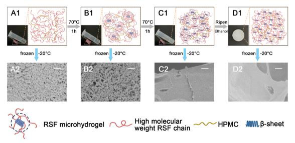
Fig. 5 Digital images and schemes of molecule chain in 6% HMWRSF/HPMC aqueous solution (A1) and its produced hydrogel at different stages (B1)-(D1). SEM images of the cross-section of those corresponding samples after lyophilization (A2)-(D2). The scale bar is 500 nm.
