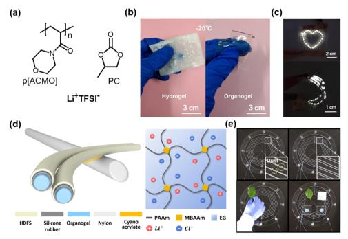
Fig. 6 Organogel-based SICs. (a) One example of organogel-based ionic conductors. (b) The organogel ionic conductor is mechanically conformable at -20 °C. (c) The organogel ionic conductor as a stretchable electrode. Reproduced with permission from ref. 61. Copyright 2019, The American Chemical Society. (d) Another example of an organogel-based ionic conductor and its components. (e) Demonstration of artificial spiderwebs. Reproduced with permission from ref. 35. Copyright 2020, AAAS.
