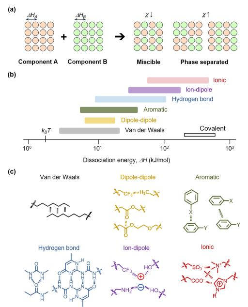
Fig. 3 Intermolecular interactions for materials design. (a) When two components are mixed, the interaction parameter  $\chi$  is a determinant factor for their miscibility. (b) A scale of the dissociation energy of diverse molecular interactions. The  $k_BT$  is thermal energy at room temperature. (c) Representative molecular moieties for different intermolecular interactions
