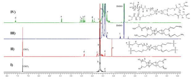
Fig. 2 <sup>1</sup>H NMR spectra of (I) the starting compound TP10k-OH, (II) the purified mesylate-terminated tetraPEG (TP10k-mesyl), (III) the purified amineterminated tetraPEG (TP10k-NH<sub>2</sub>), and (IV) the final targeted product of diol-terminated tetraPEG (TP10k-Gluco)
