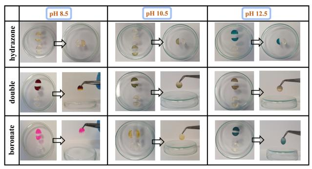
Fig. 6 Self-healing tests performed on the three hydrogel types, each prepared at three different pH values, 8.5, 10.5 and 12.5, without the addition of catalyst
