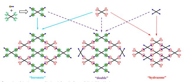
Fig. 3 Preparation of the three types of hydrogels from the four available building blocks
