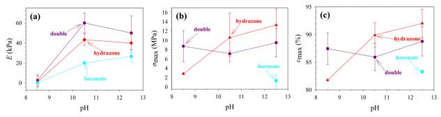
Fig. 10 Compressive mechanical properties, (a) elastic modulus, E, (b) stress at break,  $\sigma_{\text{max}}$ , and (c) strain at break,  $\varepsilon_{\text{max}}$ , of the three hydrogel types, boronate, hydrazone and double, each prepared at three different pH values, 8.5, 10.5 and 12.5
