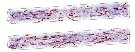
Fig. 8 Distribution of stretched segments (red cylinders) in resultant gels for s2020 (top) and Rnd (bottom) under the applied stretch  $\lambda = 5$ . The stretched segments are highlighted when consecutive segments are stretched. For the colored segments, the squared segment length is larger than 3. The dispersed beads are also shown by light blue spheres.
