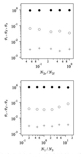
Fig. 4 Arm fractions in dangling ends  $\varphi_a$  (cross), single linkages  $\varphi_s$  (filled circle), and double linkages  $\varphi_d$  (unfilled circle) in the resultant networks for 2a2 and 1a3 systems.
