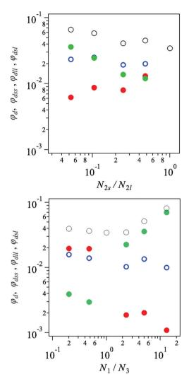
**Fig. 6** Strand fractions in double linkages formed by the arm combinations of short-short  $\varphi_{dss}$  (green filled circle), long-long  $\varphi_{dll}$  (red filled circle), and short-long  $\varphi_{dsl}$  (blue unfilled circle). The total fraction of double linkages  $\varphi_d$  (unfilled black circle) is also shown for comparison. Note that for the monodisperse case (s2020, for which  $N_{2s}/N_{2l}=N_1/N_3=1$ ), the strand length is uniform, and  $\varphi_d$  cannot be decomposed.
