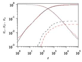
Fig. 3 Time development of number fraction of the arms. Dotted, solid, and broken curves are unreacted dangling ones  $\varphi_{a}$ , the fraction involved in single linkages  $\varphi_{s}$ , and those contributed as double linkages  $\varphi_{d}$ , respectively. Black and red curves are for 2a2-3802 and s2020, respectively.
