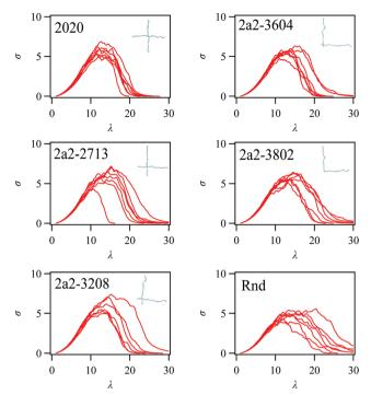
Fig. 10 Stress-stretch curves for 2a2 systems. The results from 8 independent simulation runs are shown. The results for the random network (Rnd) are also shown for comparison. The results for 1a3 systems are available in the ESI.†
