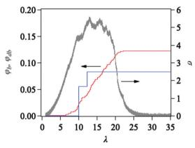
Fig. 12 Evolution of the broken strand fraction  $\varphi_b$  (red curve) during stretch for a 1a3-6505 network. Blue line indicates the broken double linkage fraction  $\varphi_{db}$ . The gray curve shows the stress for comparison.
