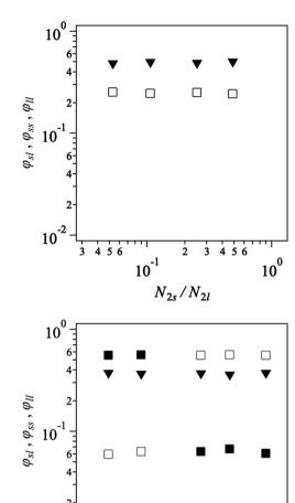
Fig. 5 Strand fractions formed with two short arms  $\varphi_{ss}$  (unfilled square), two long arms  $\varphi_{ll}$  (filled square), and short and long arms (triangle)  $\varphi_{sl}$  for 2a2 and 1a3 systems. For 2a2 systems,  $\varphi_{ll}$  and  $\varphi_{ss}$  overlap with each other; thus,  $\varphi_{ll}$  is not visible.
