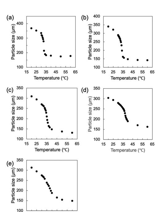
Fig. 6 Diameter of the spherical gels (a) PNIPA gel, (b) PNIPA<sub>0.9</sub>-b-PDMA<sub>0.1</sub> gel, (c) PNIPA<sub>0.8</sub>-b-PDMA<sub>0.2</sub> gel, (d) PNIPA<sub>0.7</sub>-b-PDMA<sub>0.3</sub> gel and (e) PNIPA<sub>0.8</sub>-r-PDMA<sub>0.2</sub> gel at equilibrium at certain temperature for each of them. The diameters are measured through an inverted optical microscope.
