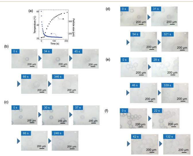
Fig. 7 (a) Variation in the diameter and temperature of the spherical PNIPA gel with time during a temperature jump from 60 °C to 20 °C, (b) – (f) Optical microscopy images in a temperature jump from 60 °C to 20 °C for (b) PNIPA gel, (c) PNIPA<sub>0.9</sub>-b-PDMA<sub>0.1</sub> gel, (d) PNIPA<sub>0.8</sub>-b-PDMA<sub>0.2</sub> gel, (e) PNIPA<sub>0.7</sub>-b-PDMA<sub>0.3</sub> gel, and (f) PNIPA<sub>0.8</sub>-r-PDMA<sub>0.2</sub> gel.
