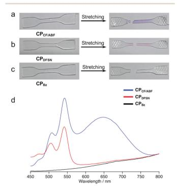
Fig. 4 Photographs of (a)  $CP_{CF/ABF}$ , (b)  $CP_{DFSN}$  and (c)  $CP_{Bz}$  films before and after fracture. (d) UV-Vis spectra of  $CP_{CF/ABF}$  (blue),  $CP_{DFSN}$  (red) and CP<sub>Bz</sub> (black) films after fracture.
