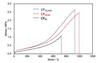
Fig. 5 Stress-strain curves of  $CP_{CF/ABF}$  (blue),  $CP_{DFSN}$  (red) and  $CP_{Bz}$ (black) films (100 mm min $^{-1}$ , 30 °C).
