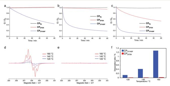
Fig. 3 Stress-relaxation behavior of  $\mathbf{CP_x}$  at (a) 120, (b) 140 and (c) 160 °C. EPR spectra of (d)  $\mathbf{CP_{CF/ABF}}$  and (e)  $\mathbf{CP_{DFSN}}$  at 120, 140 and 160 °C. (f) Dissociation ratio of CF/ABF and DFSN in CP<sub>CF/ABF</sub> and CP<sub>DFSN</sub> at 120, 140 and 160 °C.
