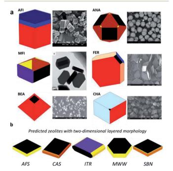
Fig. 6 The thermodynamic Wulff morphologies of different zeolites from online search. (a) Comparison between predicted and experimental zeolite morphologies. (b) The zeolites predicted to have a 2D layered morphology. All data are available at the website <a href="https://www.lasphub.com/zeolite">https://www.lasphub.com/zeolite</a>.
