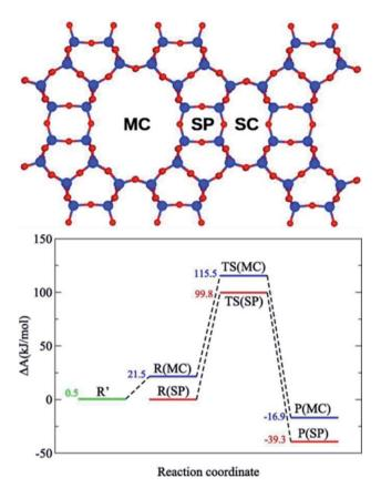
Fig. 3 Free energy profile for the methanol carbonylation reaction in MOR side pockets (SP) and main channels (MC) computed using DFT at the PBE-D2 level. Reproduced from ref. 81 with permission from Elsevier, copyright 2021.
