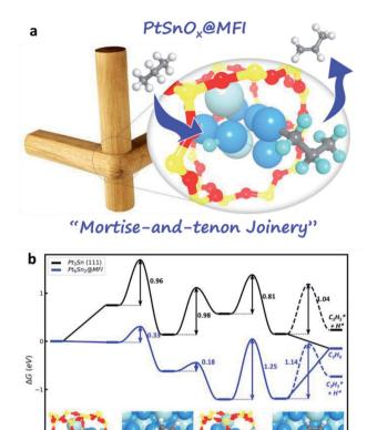
Fig. 4 Zeolite-confined subnanometric PtSn for catalytic propane dehydrogenation. (a) The sketch map of mortise-and-tenon joinery for subnanometric PtSn within MFI zeolite. (b) Gibbs free energy profiles for PDH reaction on Pt<sub>6</sub>Sn<sub>2</sub>@MFI and Pt<sub>3</sub>Sn (111) surfaces at 773 K and 1 bar propane pressure (see ref. 82)
