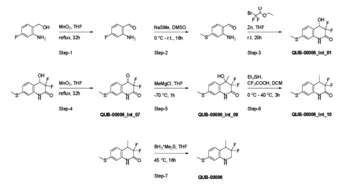
Fig. 4 Synthesis path of 3,3-difluoro-4-methyl-7-(methylsulfanyl)-1,2,3,4-tetrahydroquinoline named QUB-00006.
