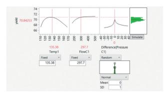
Fig. 24 Propagation of input-output uncertainties. The lack of control in pressure is simulated by including a random normal distribution in the predictive model input, generating a distribution of yield (output).
