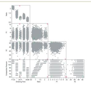
Fig. 14 Scatterplot matrix showing historical data of a manufacturing process where the optimal prediction point is shown without extrapolation control (red) and with extrapolation control (green). A boosted neural network was previously trained to predict failure and quality. The reader is referred to ref. 60 for a detailed discussion.
