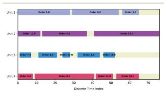
Fig. 38 Solving a MILP problem via RL to produce an optimal production schedule via the framework displayed in Fig. 37. A discrete time interval is equivalent to 0.5 days in this study.
