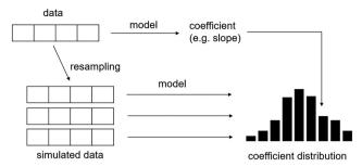
Fig. 26 Uncertainty can be estimated by comparing a model (or sample statistic) with its simulated distribution using resampling techniques. For example, the slope obtained in a linear model can be compared to a distribution of the same parameter that was generated by resampling the training data. Adapted from ref. 107 with permission.
