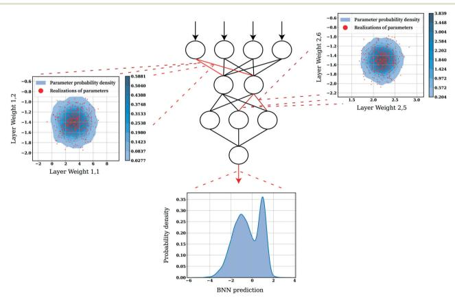
Fig. 27 Figurative description of the Bayesian approach to express modeling uncertainty in neural networks. The top two subplots show the covariance between two-parameter distributions in the first and second layers of the network, respectively. The bottom subplot demonstrates the generation of a predictive distribution by Monte Carlo sampling the parametric distributions identified via approximate Bayesian inference.
