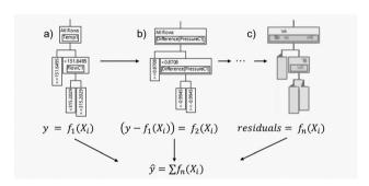
Fig. 18 By subsequently fitting the residuals of smaller trees, boosted trees can be used as discrepancy models where the first layers (a and b) capture the major variability within the data. Weaker but perhaps more interesting predictors can be identified by examining deep layers (c). Following the example used earlier, the first two layers are able to identify major drivers separately: a) flow and temperature; b) pressure stability.
