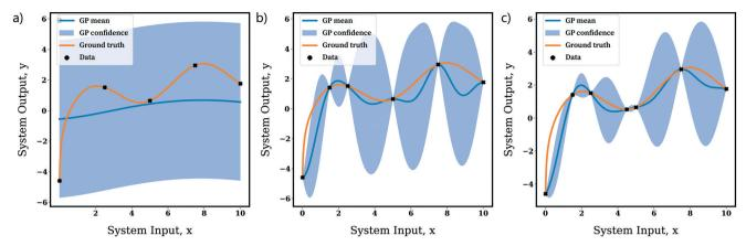
Fig. 28 Expression of a Gaussian process posterior (i.e. its mean and uncertainty predictions) for the modeling of a smooth noiseless function. The figure demonstrates the effects of an increasing number of data points: a) 5 data points, b) 6 data points, c) 7 data points. Note how as the number of data points increases, the uncertainty estimate (i.e. the 95% confidence interval) reduces and the mean GP prediction becomes a better estimate of the ground truth.
