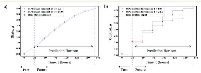
Fig. 30 Demonstration of the use of state-feedback in receding horizon MPC for online optimization of an uncertain, nonlinear fed-batch process. Optimized forecast and evolution of a) the state trajectory, b) the control trajectory (composed of piecewise constant control inputs). See ref. 158 and 159 for more information on the system detailed.
