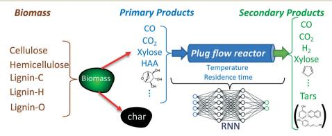
Fig. 1 Schematic of the biomass gasification process and the RNN model. The RNN models the dynamics of the freeboard region of the fluidized bed gasifier. The input to the RNN model consists of the reactor temperature and the mass fractions of 27 species provided in Table 1.
