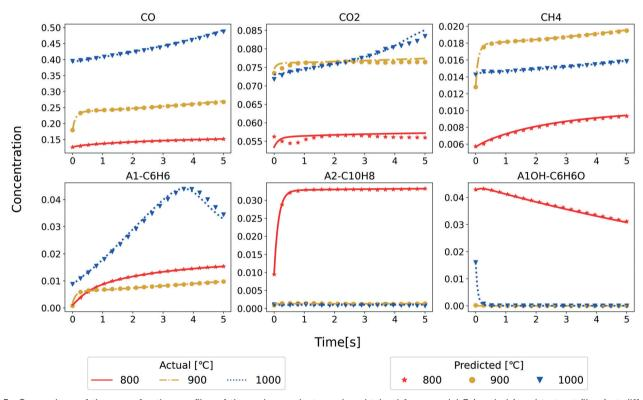
Fig. 5 Comparison of the mass fraction profiles of the major product species obtained from model 3 (symbols) and test set (lines) at different temperatures.
