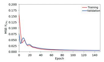
Fig. 7 Convergence of the mean square error (MSE) of the methane yield,  $Y_{CH_4}$  obtained with the ANN model consisting of 3 hidden layers with 20 neurons in each layer. The MSE for the ANN model converges after 80 epochs (iterations).
