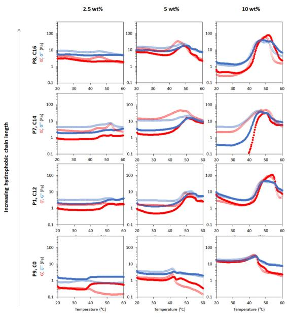
Fig. 10 Effect of hydrophobic alkyl tail length on thermo-gelation activity of emulsions as determined by a rheology temperature ramp. P9 is synthesized with mercaptoethnol, P1 with dodecanethiol, P7 with tetradecanethiol and P8 with hexadecanethiol, leading to alkyl chain lengths of 0, 12, 14, and 16 C atoms, respectively. G' is shown in red and G'' is shown in blue. Full rheograms showing the Y-axis region < 0.1 Pa for P7 at 10 wt% are shown in Fig. S15.†
