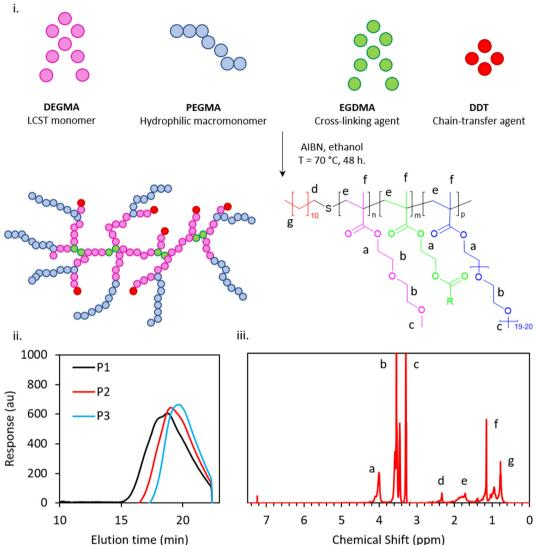
Fig. 1 Free radical polymerisation of PDEGMA-PEGMA-EGDMA-DDT and theoretical structure of the branched copolymer surfactant (BCS) (i), exemplar GPC chromatogram of P1-3 (ii) and exemplar <sup>1</sup>H NMR spectrum (iii).
