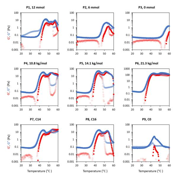
Fig. 12 Temperature ramp rheology of 20 wt% BCS solutions in D<sub>2</sub>O. Filled and open circles show the heating and cooling cycles, respectively.
