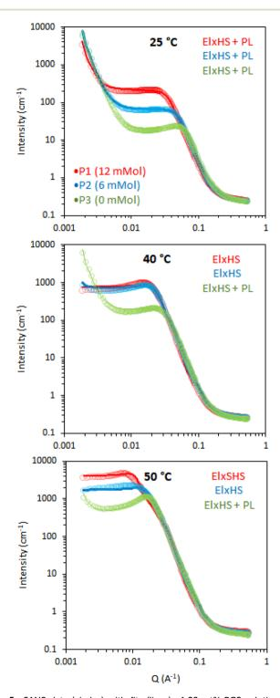
Fig. 5 SANS data (circles) with fits (lines) of 20 wt% BCS solutions in  $D_2O$  with variation of cross-linking and temperature. Legend inset shows sample ID and cross-linker feed. Models used to fit data are inserted at the top right. El is an ellipsoid form factor, HS and SHS are hard sphere and sticky hard sphere structure factors, respectively, whilst  $\times$  and + are mathematical operators. PL is a power law with a  $q^{-4}$  decay.
