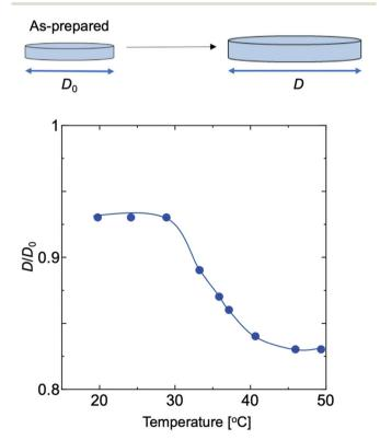
Fig. 6 Temperature dependence of the degree of swelling in water of polymer gels composed of EO2 prepared by adding 50 times the crosslinker to the initiator (750 mM).
