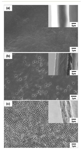
Fig. 2 SEM images of (a) pristine poly(DABA-co-ABA), (b) porous poly (DABA-co-ABA)-30%, and (c) porous poly(DABA-co-ABA)-50% film. SEM images of cross-section of films are inset.
