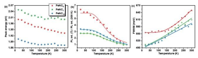
Fig. 5 Temperature-dependent PL (a) emission peak energy, (b) peak intensity, and (c) FWHM of PeNC<sub>0</sub>, PeNC<sub>1</sub>, and PeNC<sub>10</sub>.
