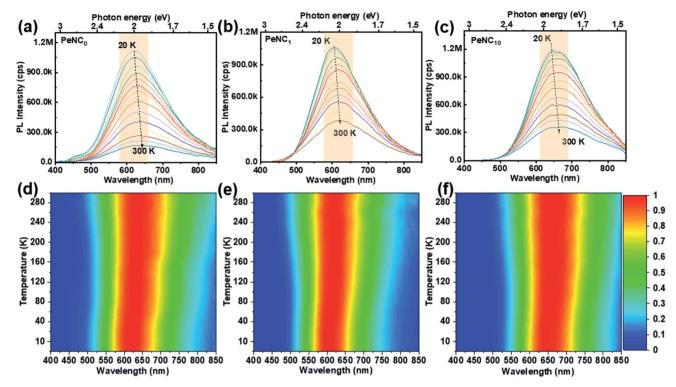
Fig. 4 Temperature-dependent PL spectra of (a) PeNC $_0$  ( $\lambda_{ex} = 275$  nm), (b) PeNC $_1$  ( $\lambda_{ex} = 330$  nm), and (c) PeNC $_1$ 0 ( $\lambda_{ex} = 330$  nm) from 20 to 300 K. Normalized PL intensity mapped with the emission wavelength and temperature for (d) PeNC $_0$  (e) PeNC $_1$ 1, and (f) PeNC $_1$ 2.
