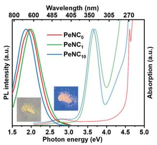
Fig. 3 UV-Vis absorption and PL spectra of PeNC $_0$  ( $\lambda_{ex}=275$  nm), PeNC $_1$  ( $\lambda_{ex}=330$  nm), and PeNC $_1$ 0 ( $\lambda_{ex}=330$  nm) with nanocrystals in the powder form. Photographs showing the PeNC $_1$  powder sample under room illumination (left) and UV irradiation (right).
