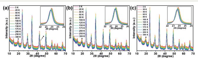
Fig. 2 LT-XRD patterns of (a) PeNC<sub>0</sub>, (b) PeNC<sub>1</sub>, and (c) PeNC<sub>10</sub> in the temperature range from 5–300 K. Peaks indicated as  $\star$  and  $\bullet$  are from the X-ray window materials of the cryostat and from the Cu sample holder, respectively.
