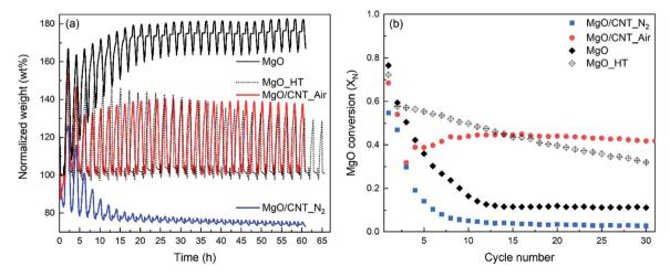
Fig. 3  $CO_2$  capture performance of MgO-based sorbents for 30 cycles of carbonation—dissociation measured by TG-DSC. (a) Normalized weight (wt%) profiles and (b) MgO conversion ( $X_N$ ). Weight profiles are normalized according to each weight of pristine MgO-based sorbents.
