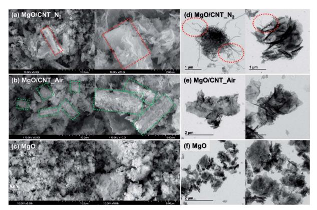
Fig. 2 SEM and TEM images of pristine MgO sorbents. SEM images of (a) MgO/CNT\_N<sub>2</sub>, (b) MgO/CNT\_Air, and (c) MgO samples, and TEM images of (d) MgO/CNT\_N<sub>2</sub>, (e) MgO/CNT\_Air, and (f) MgO. Dotted areas in red and in green indicate CNT with MgO flakes, and tubular-shaped MgO flakes without CNT, respectively.
