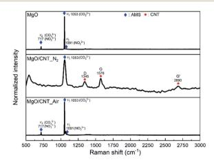
Fig. 5 Raman spectra of MgO-based sorbents after 30 cycles of carbonation–calcination reactions.
