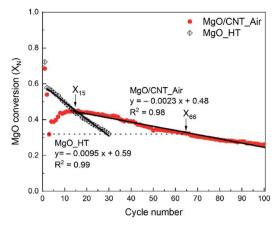
Fig. 4  $CO_2$  capture performance of MgO\_HT (30 cycles) and MgO/CNT\_Air (100 cycles) in MgO conversion ( $X_N$ ) by TG-DSC. Linear regressions of performance decay are given.
