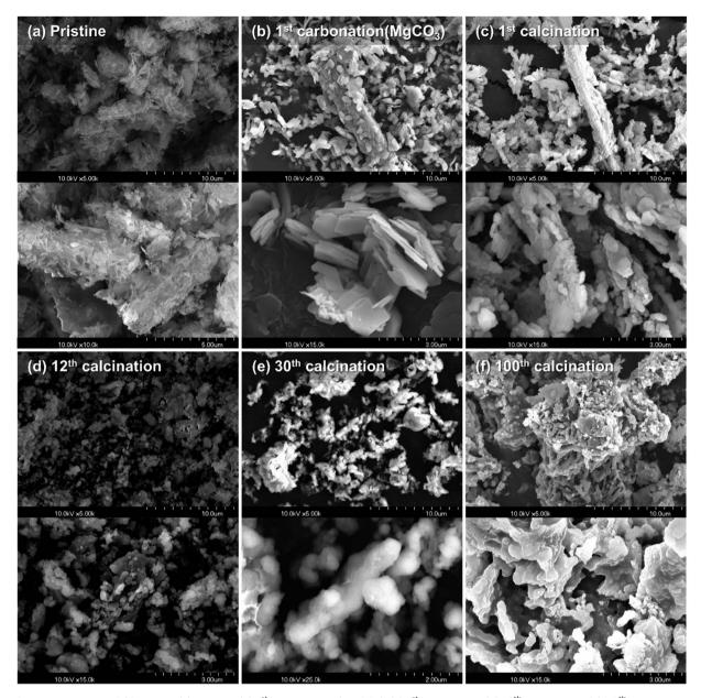
Fig. 6 SEM images of MgO/CNT\_Air: (a) pristine, (b)  $1^{st}$  carbonation (MgCO<sub>3</sub>), (c)  $1^{st}$  calcination, (d)  $12^{th}$  calcination, (e)  $30^{th}$  calcination, and (f)  $100^{th}$  calcination.
