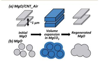
Fig. 8 Simplified schemes of morphological evolution during carbonation-calcination reaction in MgO/CNT\_Air and MgO.
